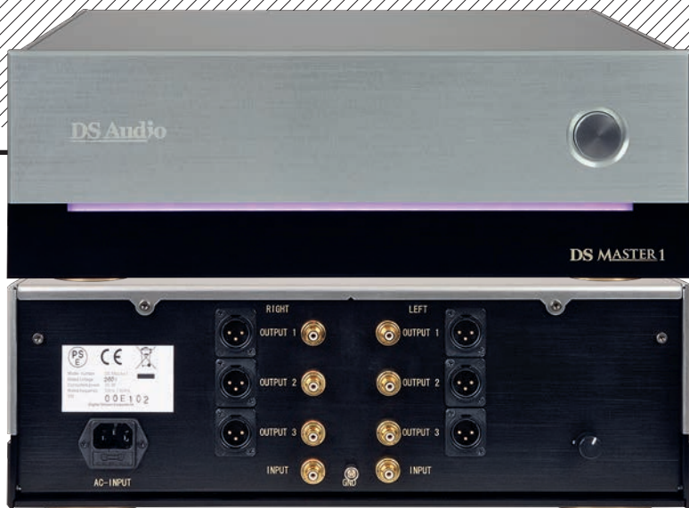
ABOVE: Front [top] and rear [bottom] views of the massive Master 1 PSU/equaliser. The pick-up's internal LED is powered via the R- and L- pins while the output is returned via R+ and L+ using the 'Input' RCAs. The three equalised outputs, on RCAs and XLRs, offer progressively steeper LF roll-offs [see Lab Report, adjacent]
